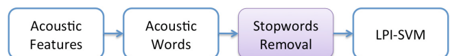
Figure 1: Diagram of the LPI-SVM based unstructured audio information retrieval system along with the proposed stopword removal process.
