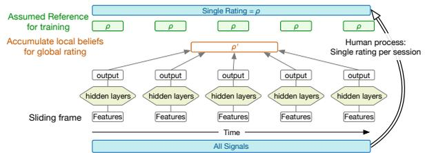
Figure 1: During training, local reference is assumed to be equal to global as denoted by the green row of  $\rho$ . During testing the mean rating is assigned as the estimated session-level rating  $\rho'$ .
