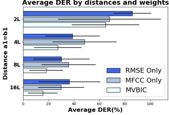
Fig. 2. Average DER by distances of interfering speakers from primary speakers.
