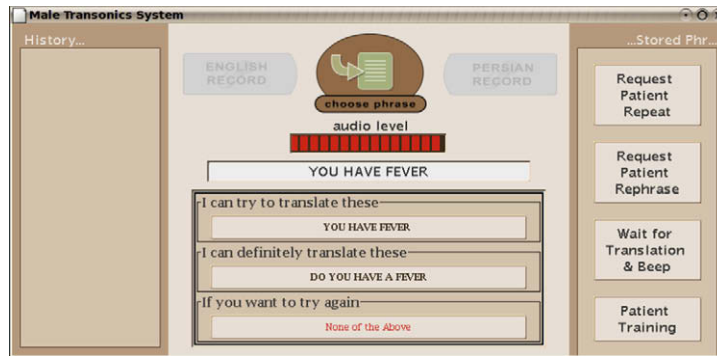
Fig. 3. Transonics system screen GUI. After speaking, the user (doctor) can choose one of several hypotheses presented on the GUI.
