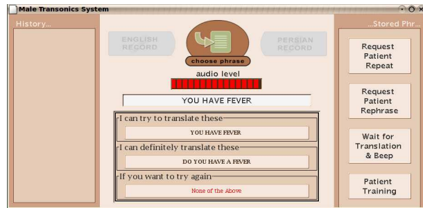
Figure 1: Transonics system screen GUI. After speaking, the user (doctor) can choose one of several hypotheses presented on the GUI.
